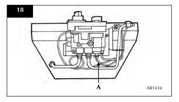
• Undo the mag unit retaining nut at the back of the control valve behind the thermocouple nut
